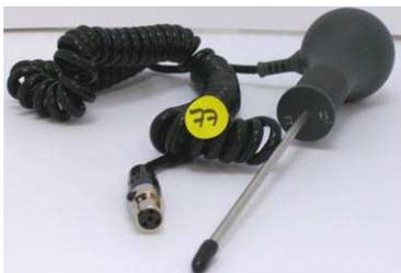
SONDE THERMOCOUPLE K.
